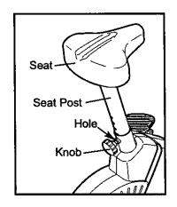
Next, slide the seat post up or down and align one of the adjustment holes in the seat post with the indicated hole in the Frame. Insert the knob into the frame and the seat post, and turn the knob clockwise until it is tight. Make sure that the knob is inserted through one of the adjustment holes in the seat post.
